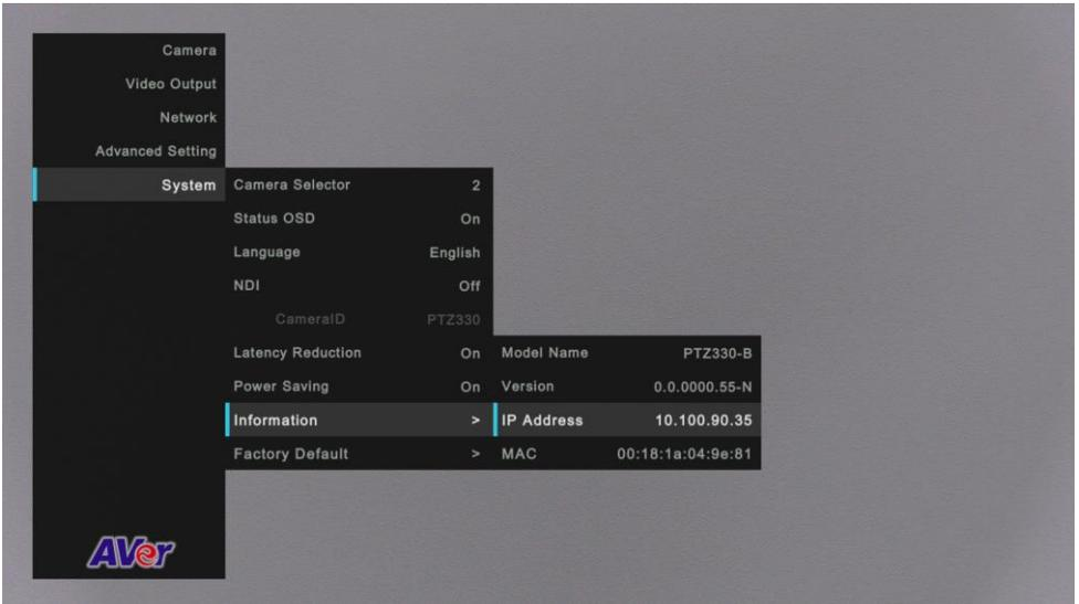
2. Open the browser and enter the IP address of the camera. The PC/laptop is required an internet access.
