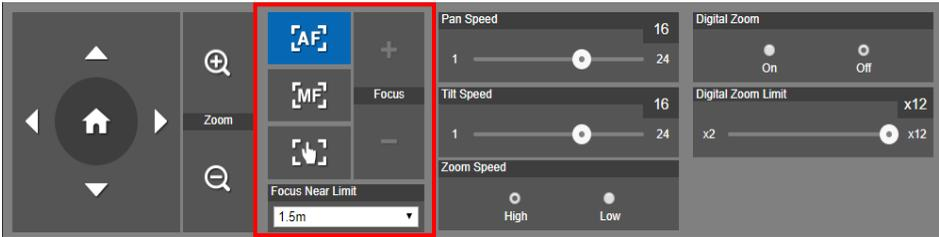
**One push focus:** By clicking the button to adjust Lens focus automatically once.
