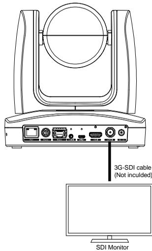
**[Note]** HDMI and 3G-SDI monitors can be connected to camera and output live video simultaneously; Assuming HDMI monitor is well connected before the camera turned on, the OSD menu will be displayed on HDMI monitor in default.”
