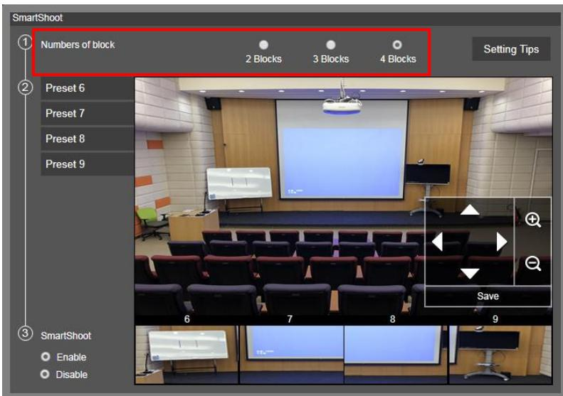
2. Set the preset positions in order (preset 6 to preset 9). Use direction control panel to move the camera to wanted position and select “save” to save the preset position. And, a snapshot of the preset image will show at corresponding image display box. Repeat the step to set another preset position.
