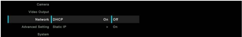
3. After turn the DHCP on, the user can go to **System > Information** to view IP address.
